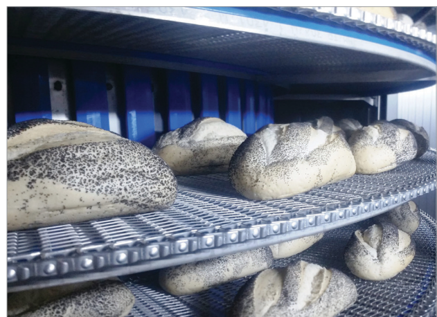
Spiral Freezer processing bread loaves for bakery production
