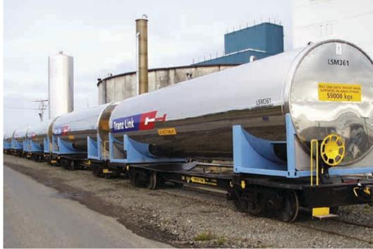
With frames and loadings rated for standard buggy sizes, the tankers are engineered to easily withstand forces transmitted through shunting and cornering. The design incorporates band panels to enable easy replacement. They can also be equipped with CIP and product handling requirements such as heating, cooling, insulation or power to ensure the product gets to its destination in the same condition it left.
