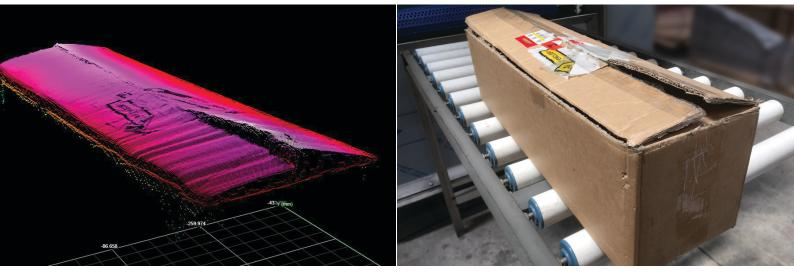
^ The UBC scans a damaged box and adjusts accordingly to accurately cut it open.
