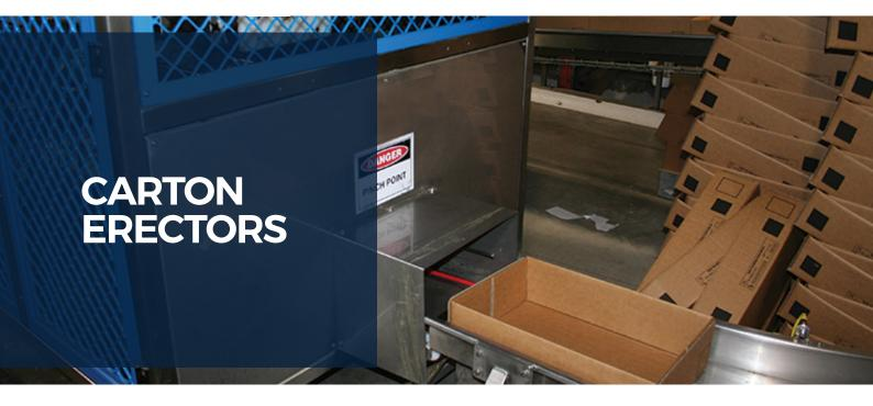
For the meat export, horticulture and food industries, carton erectors are precision designed, engineered and manufactured from stainless steel with industrial nylon components.
